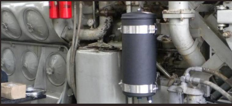
The water filter unit is installed on the structure of the engine of the general motor. Installation external takes approximately 4 hours.
